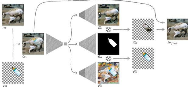
Figure 3: *Method overview.* The network consists of one encoder and three decoders. The top and bottom decoder branches reconstruct the background image and the overlaid visual motif, respectively. The middle branch estimates the mask of the visual motif. The final output is generated by using the mask to select pixels from either the input image or the reconstructed image.
